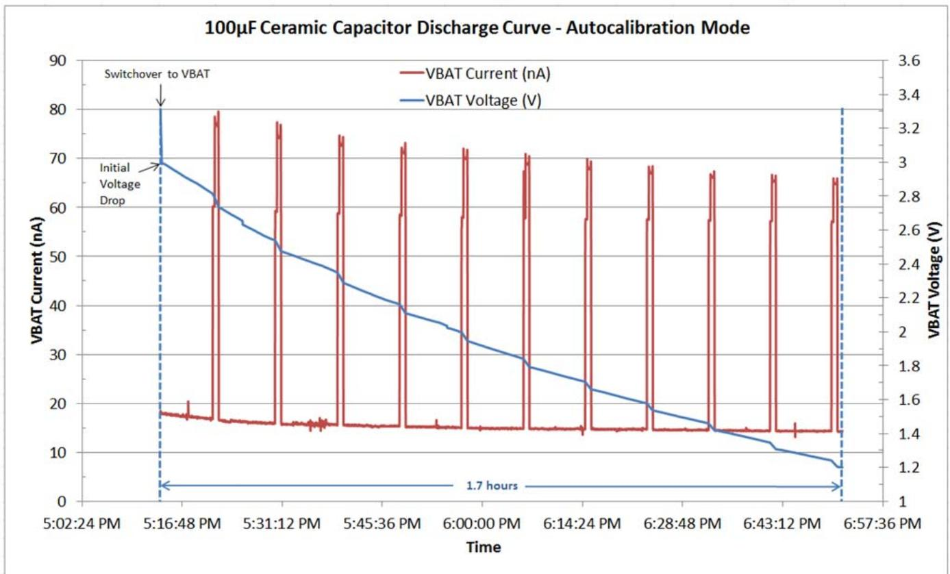
**Figure 6 – Autocalibration Mode Backup Example**
