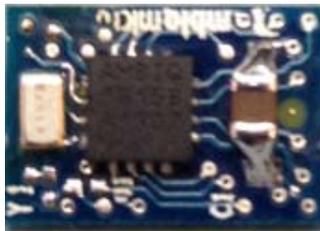
**Figure 7 – ABX8XX RTC Backup Module on FR4 Substrate**
