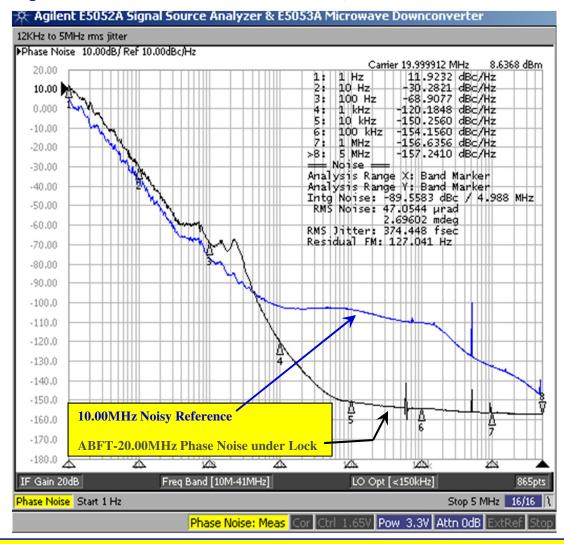
If ABFT is driven from a Noisy 10.00MHz reference, the intrinsic phase noise of the ABFT device will take over; starting at about 1kHz offset and will be typically better than -150dBc/Hz @ 10kHz away from the carrier. This will yield better than 0.50 ps rms jitter over 12kHz to 20MHz BW, *regardless of the input reference noise*
