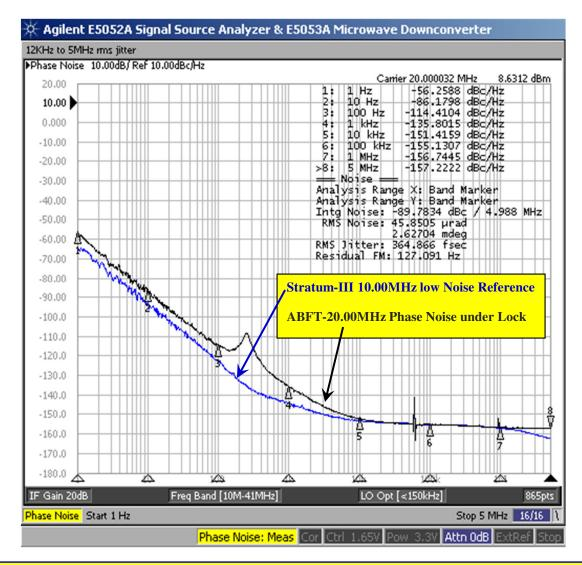
If ABFT Translator is driven with an Ultra low noise 10.00MHz reference, the intrinsic phase noise of the Translator; starting at 10kHz offset will typically be better than -150dBc/Hz
